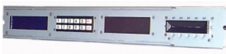
This is the front view of the display, keypad, blank, and cardreader components mounted to the faceplate.
